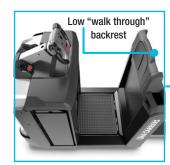
The wide platform has a low and narrow backrest, allowing the driver to quickly walk through the truck without hitting their elbows.
